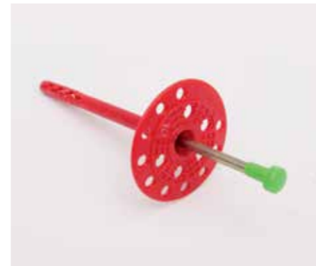
Kalekim Anchor with Steel Nail It is a mechanical fitting piece which is used to fix the Kale Thermal Insulation Boards to the reinforced concrete and hard surfaces. Steel nail is particularly preferred in Stone Wool insulation applications.
