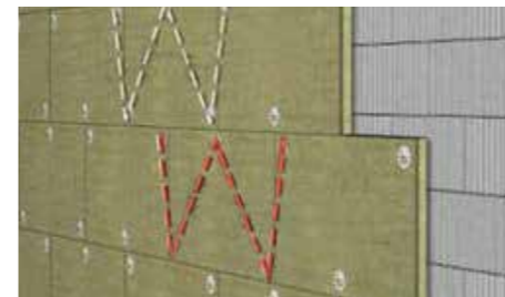
No need to block corners since thermal expansion is too low. Fix the anchors in "W" shapes
